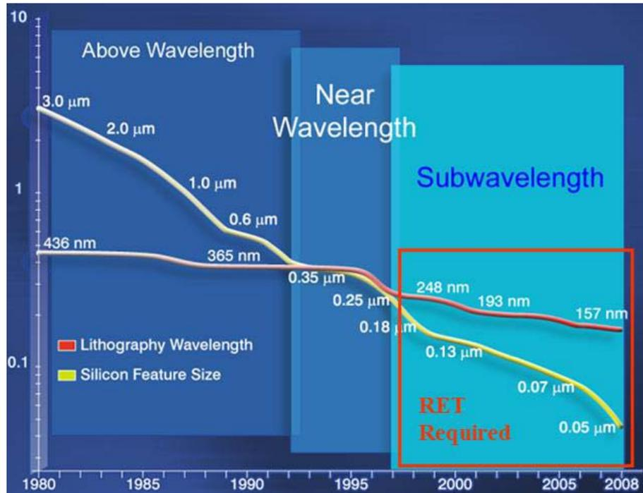
**Figure 1A – The sub-wavelength gap**
