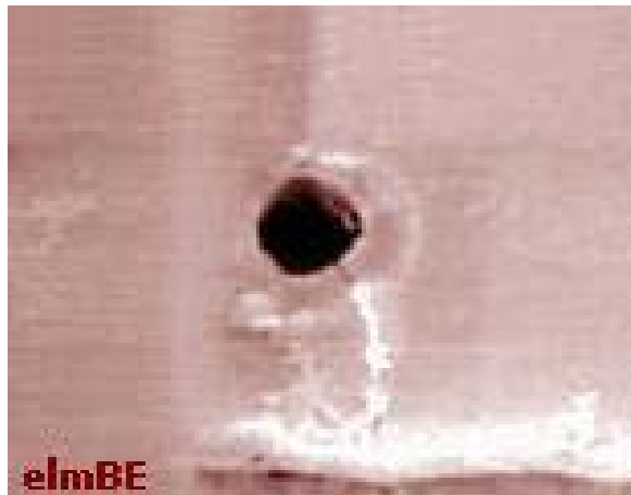
Figure 6 - Photo of an ESD-induced Oxide Breakdown
